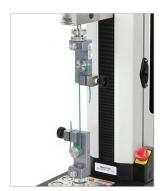
Wire tensile testing
