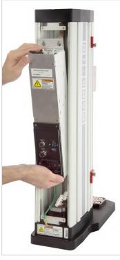
Removing the electronics module
