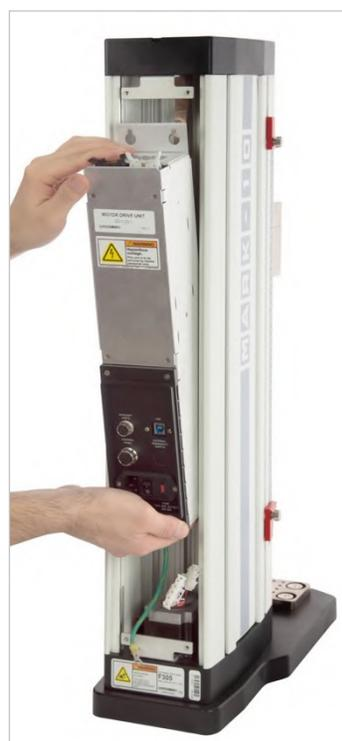
Removing the electronics module
