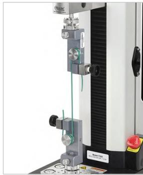
Wire tensile testing
